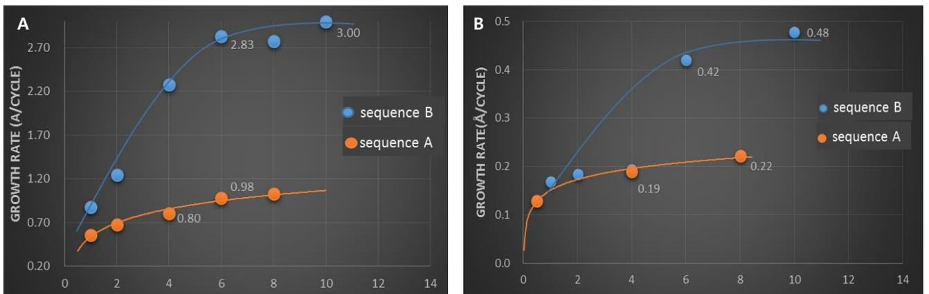
Figure 2. The growth rate (GR) of SiN films versus dosing times of silicon precursors (A – Si<sub>2</sub>Cl<sub>6</sub>, B – SiBr<sub>4</sub>) in amine catalyzed PEALD-SiN (blue dots) and normal PEALD-SiN (orange dots) processes.
