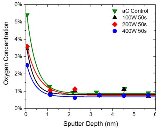
Figure 1: Oxygen depth profiles determined by XPS depth profiling of 100 nm aC films deposited on Si wafers, both treated (100W 50s black triangles, 200W 50s red diamonds, 400W 50s blue circles) and untreated (green triangles). The initial surface scan, i.e., zero sputter depth, shows higher oxygen concentration than that obtain after ~1-2 nm Ar sputtering into the aC film. Plasma treatments reduce surface oxygen content but do not inhibit partial reoxidation when exposed to air.
