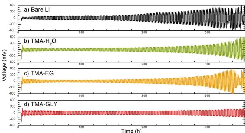
**Figure 1.** (a-d) Galvanostatic cycling of ALD and MLD coated Li-Li symmetric cells
