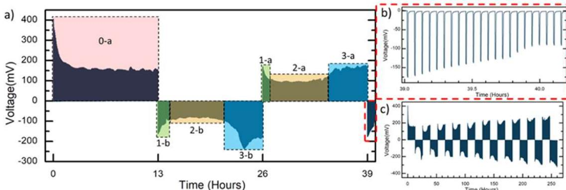
**Figure 3.** a) First few cycles of GITT data for bare Li outlining an envelope voltage pattern. b) Cells are cycled using a 15s current pulse at a density of 5 mA cm<sup>-2</sup> followed by a rest period of 3 minutes until a capacity of 5 mAh cm<sup>-2</sup> is attained.
