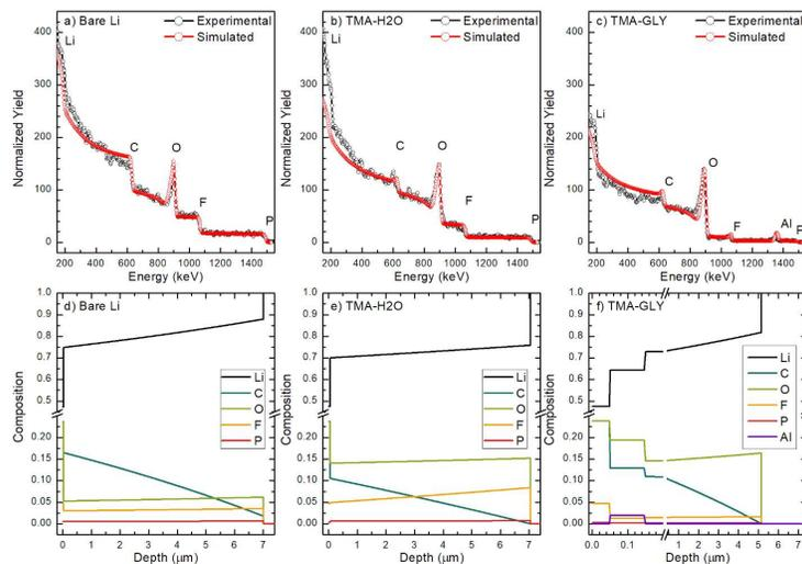
**Figure 2.** (a, d) Rutherford Back Scattering spectra and calculated depth profile for bare Li, (b, e) TMA-H<sub>2</sub>O coated Li, and (c, f) TMA-GLY coated Li following galvanostatic cycling.
