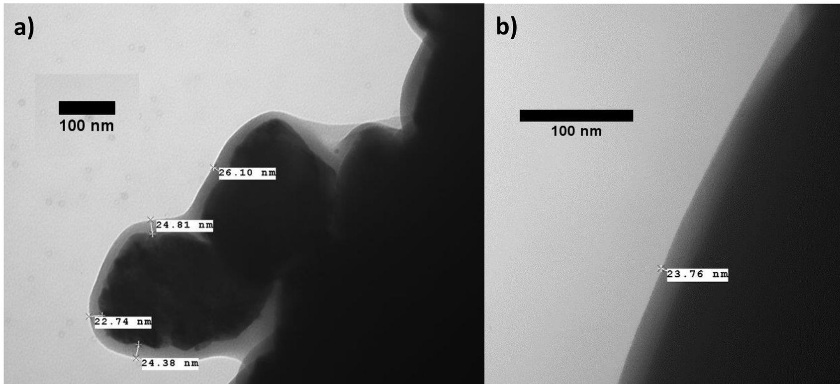
**Figure 1.** a) 60 cycles of polyamide MLD on  $\text{ZrO}_2$  nanoparticles at 67 °C. b) 60 cycles of polyamide MLD on large cellulose particles with diameters of  $\sim 200 \mu\text{m}$  at 67 °C. Thickness of polyamide film is in agreement with a MLD growth rate of 4 Å/cycle and consistent on varying sizes and compositions of particles.
