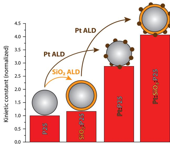
**Figure 1:** Kinetic constants for the photocatalytic degradation of Acid Blue 9 using different catalysts deposited in a fluidized bed ALD reactor. The Pt:SiO<sub>2</sub>:P25 catalyst (3 wt% SiO<sub>2</sub>, 0.34 wt% Pt) was developed by applying SiO<sub>2</sub> ALD followed by Pt ALD.
