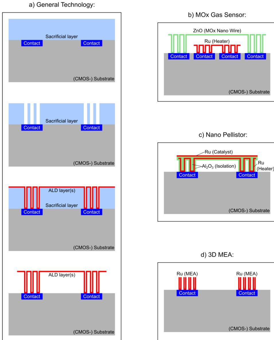
**Fig. 1:** Cross section (not on scale) of the technology and the three applications.
