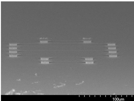
**Fig. 2:** SEM-image of a 350 nm wide and 150 µm long Ru nano wire.
