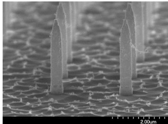
**Fig. 3:** SEM-image of 3D MEA with a tip diameter of 100 nm.
