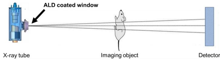
**Figure 1:** Schematic showing the position of an ALD-coated window in an imaging setup.
