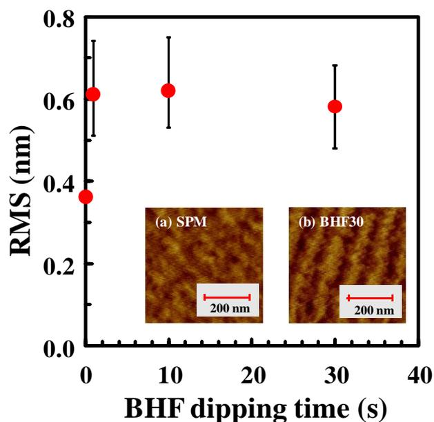
**Fig. 1** The surface roughness of  $\beta$ -Ga<sub>2</sub>O<sub>3</sub> substrates as a function of the time of BHF treatments. Insets show AFM images of  $\beta$ -Ga<sub>2</sub>O<sub>3</sub> substrates cleaned by (a) SPM 5min and (b) BHF 30 min. The RMS increased rapidly by BHF treatment from 0.35 to 0.6 nm. The RMS values showed a same values (~0.6 nm) regardless of time of BHF treatment.
