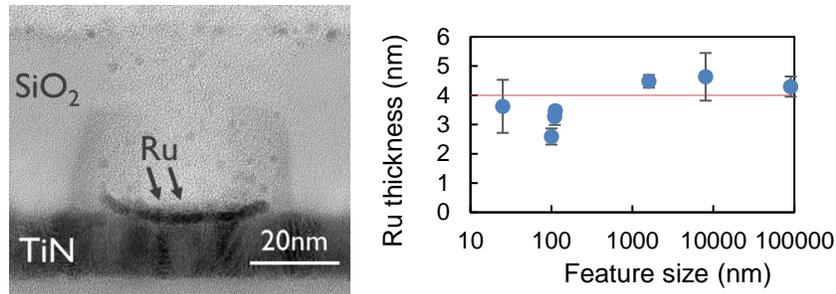
Figure 1: a) Transmission Electron Micrograph (TEM) of Ru ASD in a 25nm feature, b) Ru thickness measured in nanopattern features of different sizes. Each thickness is measured after 83 Ru ALD cycles corresponding to 4nm Ru on blanket TiN substrates (red line).
