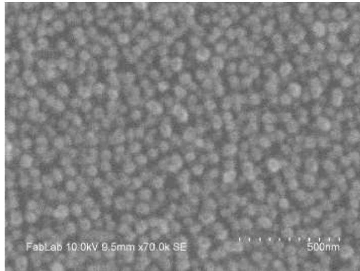
Figure 1. Scanning electron image of the reduced NiO thin-film. Reduction is performed using molecular hydrogen balanced with argon at 400°C.
