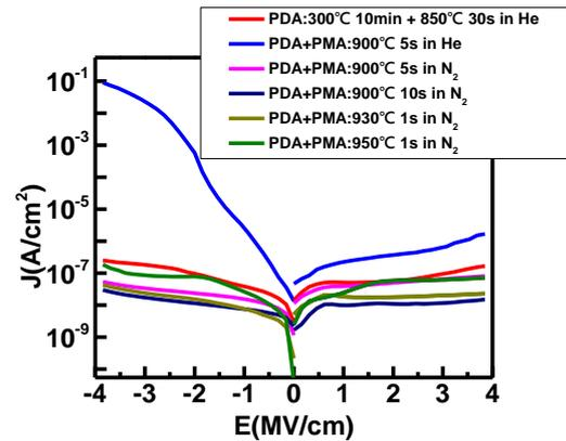
Figure 4. J-E characteristics of  $Al_2O_3$ (5nm)/ $Y_2O_3$ (1.5nm)/(In)GaAs(001) after different PMA conditions. All the samples have undergone the same PDA at 850°C 30s in He prior to ALD-TiN deposition.
