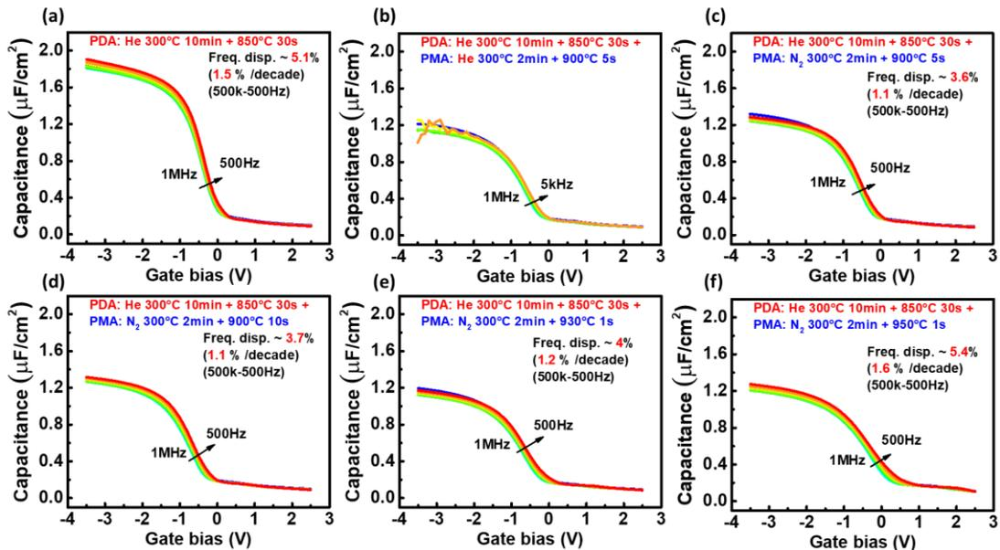
Fig. 5. C-V characteristics of  $Al_2O_3$ / $Y_2O_3$ /(In)GaAs(001) (a) without PMA, (b) with PMA at 900°C 5s in He (c) with PMA at 900°C 5s in  $N_2$  (d) with PMA at 900°C 10s in  $N_2$  (e) with PMA at 930°C 1s in  $N_2$  and (f) with PMA at 950°C 1s in  $N_2$ . All the samples have undergone the same PDA at 850°C 30s in He prior to ALD-TiN deposition.
