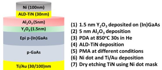
Fig. 2. ALD-TiN/ $Al_2O_3$ / $Y_2O_3$  MOSCAP structure on p-(In)GaAs (001) and MOSCAP fabrication process flow
