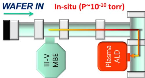
Fig. 1. Schematic showing part of our UHV multi-chamber growth/analysis system.
