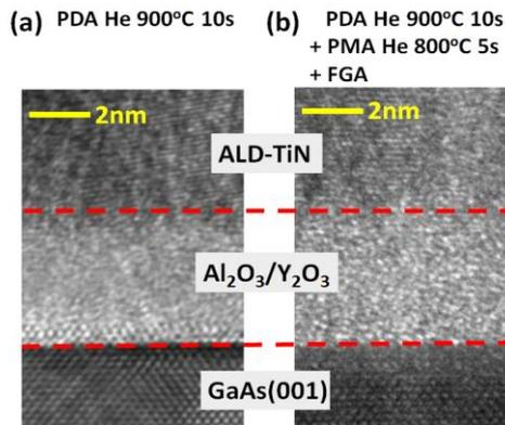
Fig. 3. cross-section TEM images of  $Al_2O_3$ (5nm)/ $Y_2O_3$ (1.5nm)/(In)GaAs(001) (a) PDA of 900°C 10s in He followed by 30nm ALD-TiN deposition and (b) further PMA of 800°C 5s in He and forming gas annealing
