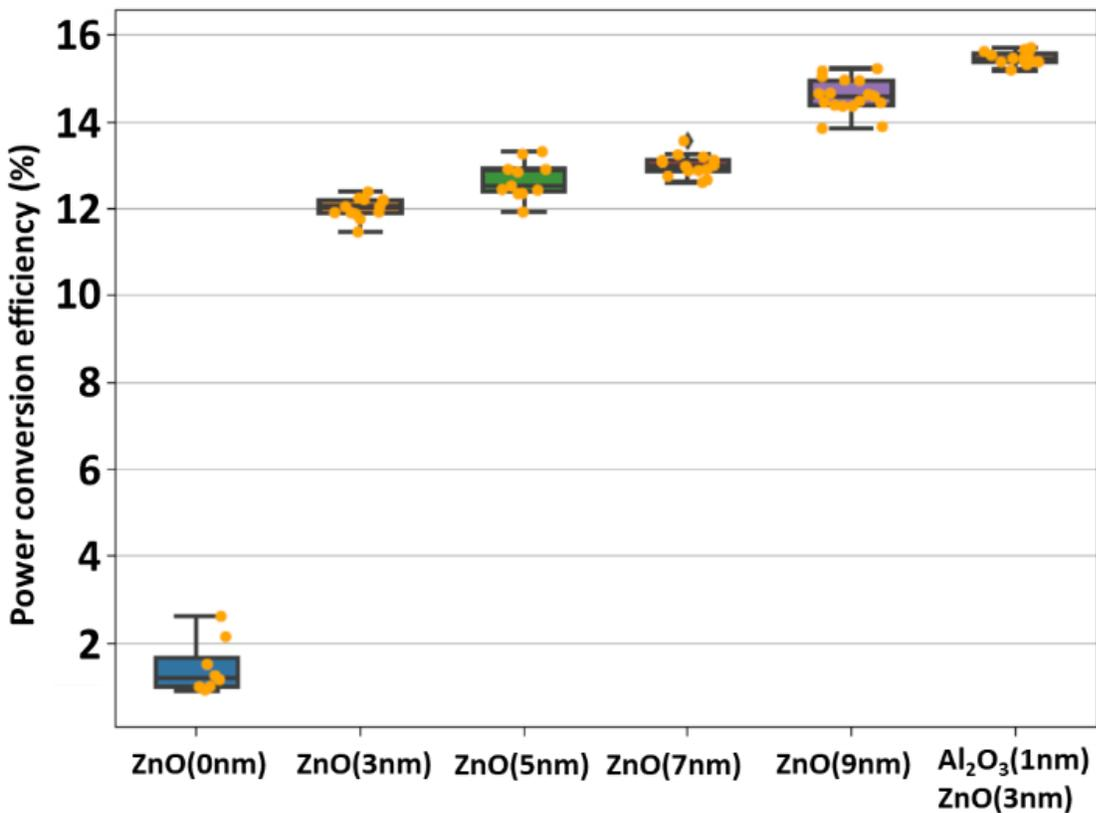
Figure 1. Comparison perovskite solar cell performance with different thicknesses of ZnO
