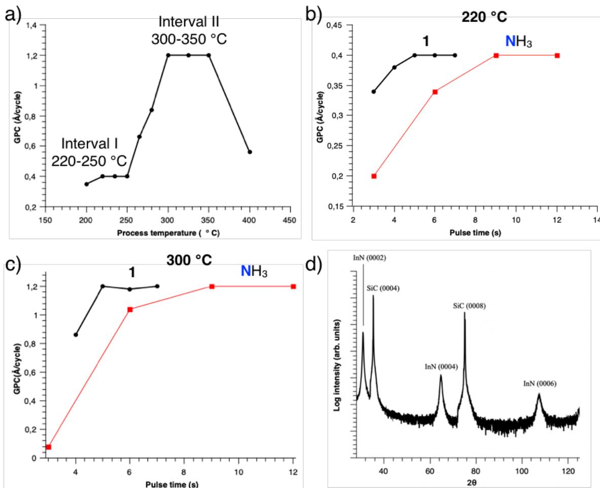
**Figure 2.** a) The growth dependence on process temperature using **1** and  $\text{NH}_3$  plasma. b) The growth per cycle behavior of **1** and  $\text{NH}_3$  pulses deposited at 220 °C. c) The growth per cycle behavior of **1** and  $\text{NH}_3$  pulses deposited at 300 °C. d) XRD of InN on 4H-SiC (0001) using **1** and  $\text{NH}_3$  plasma at 325 °C showing epitaxial InN along the c-axis.
