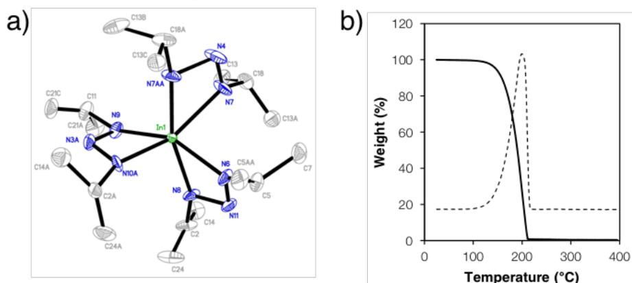
**Figure 1.** a) ORTEP drawing of **1** with thermal ellipsoids at the 50% probability level. All hydrogen atoms were removed for clarity. b) Thermogravimetric analysis of compound **1**.
