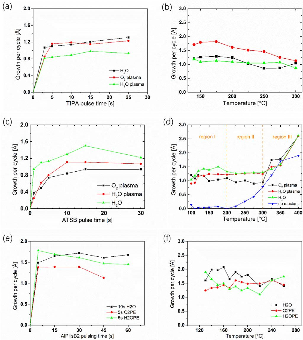
Figure 1 Saturation behavior of ALD processes using (a) TIPA, (c) ATSB and (e) AiP1sB2 as precursors with 5s co-reactants and temperature windows achieved by (b) TIPA, (d) ATSB and (f) AiP1sB2 as precursors.
