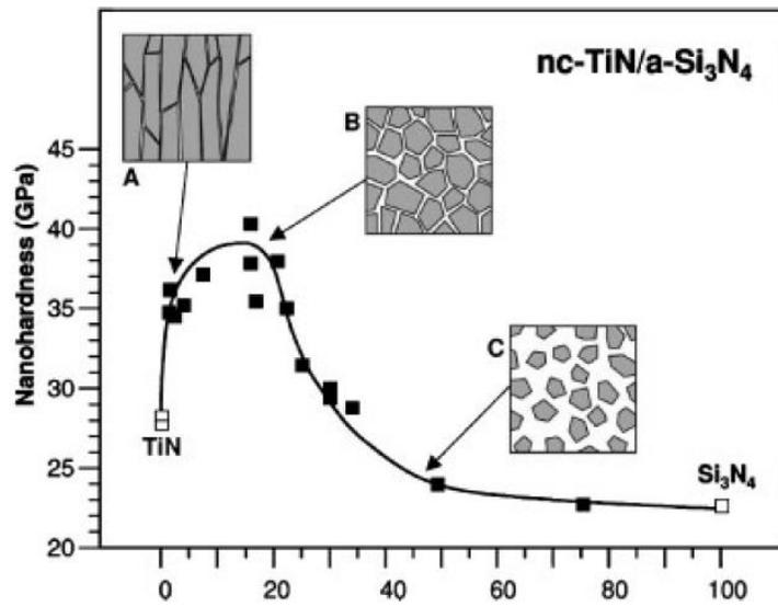
Figure 2. Hardness of nanocrystalline-TiN/amorphous-Si<sub>3</sub>N<sub>4</sub> as a function of Si-nitride fraction. Inset illustrates the
