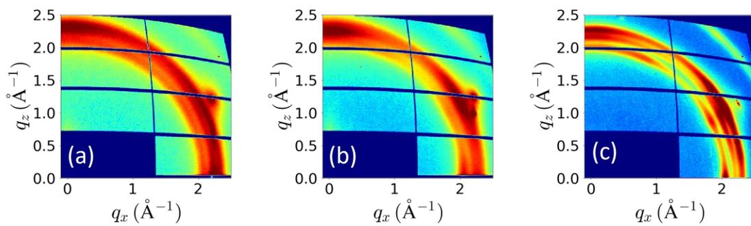
FIG 1. *Ex situ* GIWAXS pattern for  $\text{In}_{.62}\text{Al}_{.38}\text{N}$  superlattices in which each ALEp supercycle consisted of (a) 2/21 (b) 3/30 (c) and 9/90 AlN/InN subcycles. The degree of texturing increases with the superlattice period.
