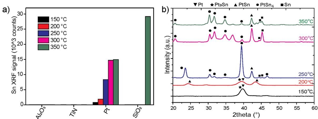
**Figure 1. a)** *Ex situ* XRF data showing the selective decomposition of TDMASn on Pt thin films. The TDMASn was pulsed into the reactor in discrete pulses, followed by a pumping step after each exposure. **b)** XRD patterns showing the formation of different Pt-Sn alloys after the TDMASn introduction to Pt.
