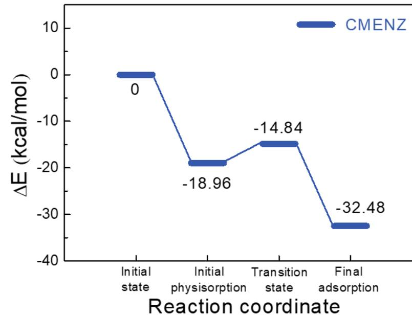
Figure 1. Change of energy calculated by DFT
