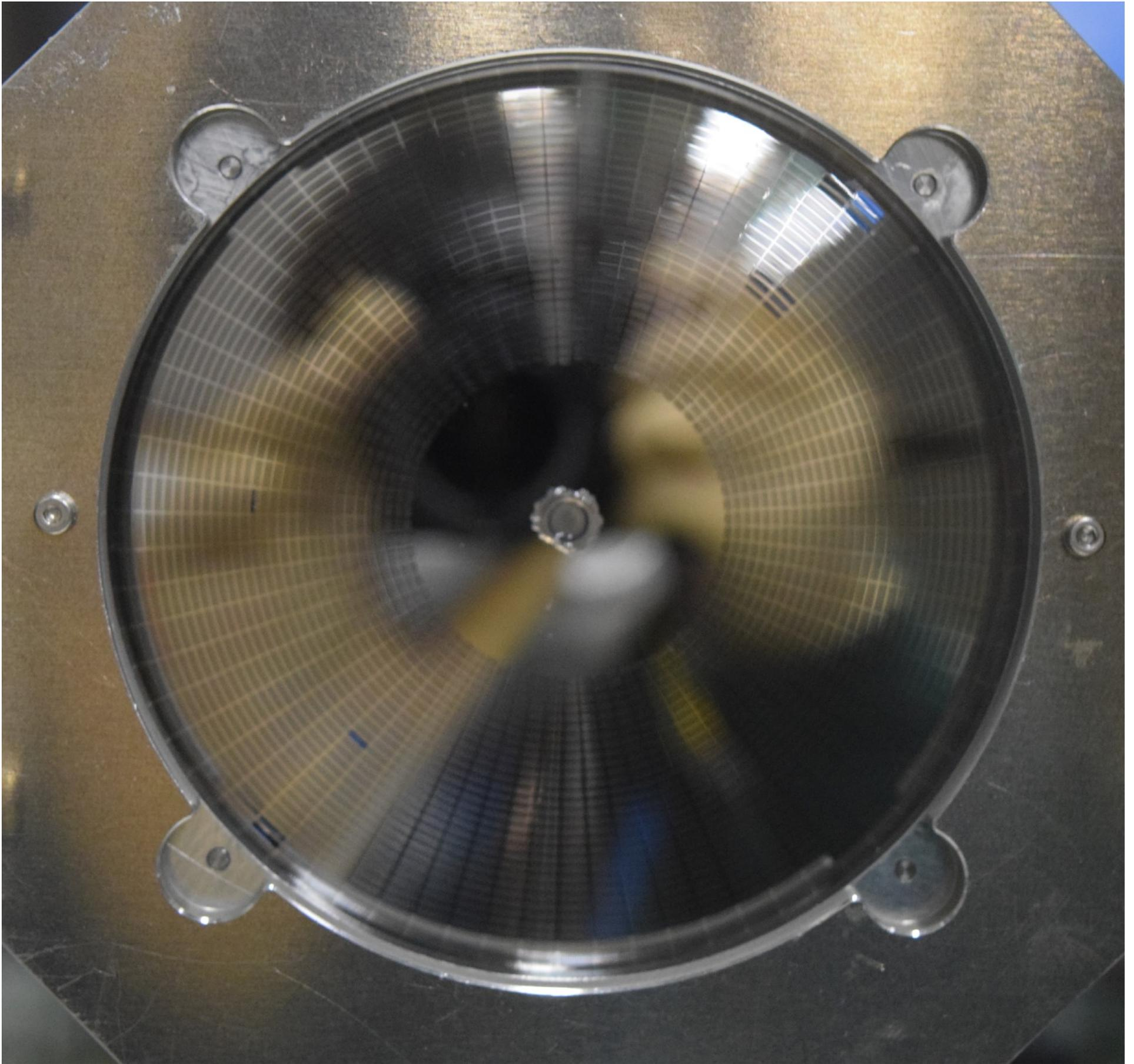
**Fig.1 A photo of an engineering model of the Pt-coated MEMS X-ray telescope for the GEO-X mission.**
