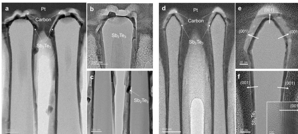
**Figure 3.** Cross-sectional TEM images of a  $\text{Sb}_2\text{Te}_3$  film on a three-dimensional contact hole structure (a-c) without, and (d-f) with an a-GeTe buffer layer.
