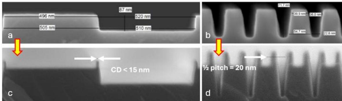
Figure 1. Cross-sectional images of a 90 nm tall a-Si line defined by EBL on a 300-mm wafer after pattern transfer and mask removal a) 500 nm width and 500 nm half-pitch; (b) 40 nm width and 40 nm half-pitch; (c) feature shown in a) after APS, depicting a CD < 15 nm and (d) feature shown in b) after APS, demonstrating a half-pitch of 20 nm. These results confirm that the CD of fins is independent of the original line width.
