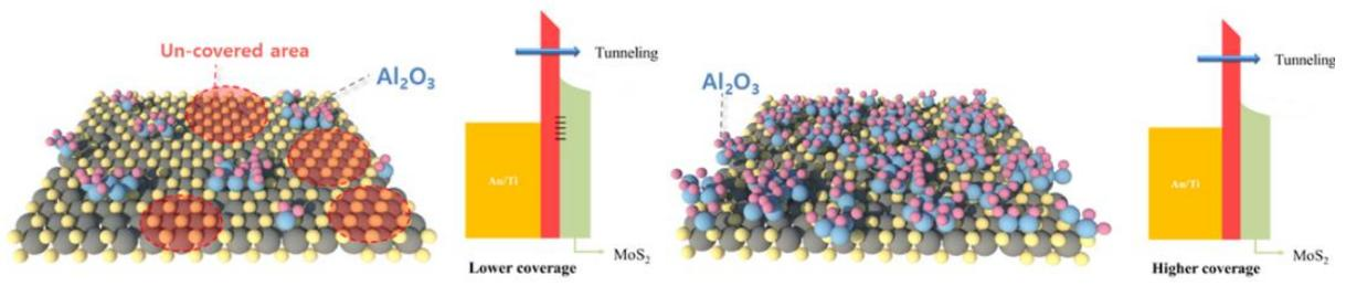
Fig 1. Schematic of different Al<sub>2</sub>O<sub>3</sub> coverages on MoS<sub>2</sub> films and their band structures
