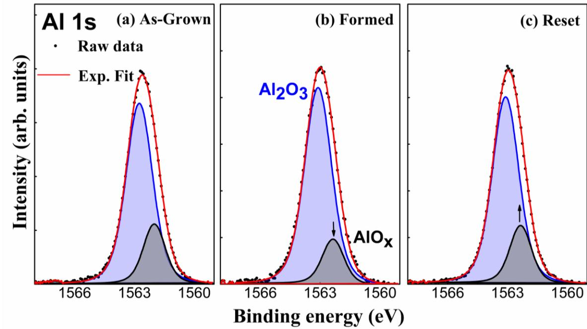
Fig. 1: Al 1s core level spectra obtained by HAXPES on As-grown, Formed and Reset states of the TaN/TiTe/ $\text{Al}_2\text{O}_3$ /Ta CBRAM stack.
