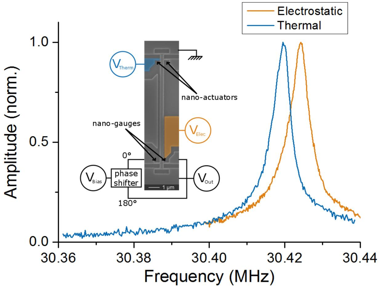
Fig. 1: Typical frequency response of one nanoresonator of the array measured with electrostatic (orange) or thermal (blue) actuation. Due to Joule heating the thermal drive induces a downshift. Inset: Setup with SEM picture of a typical NEMS. The color highlights the actuation schemes being compared.
