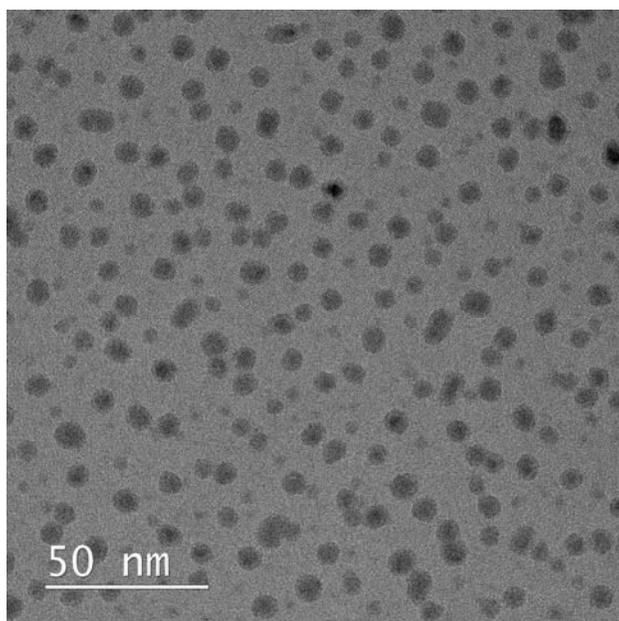
Figure 1: Ex-situ TEM image of ALD cobalt nanoparticles obtained after 250 cycles
