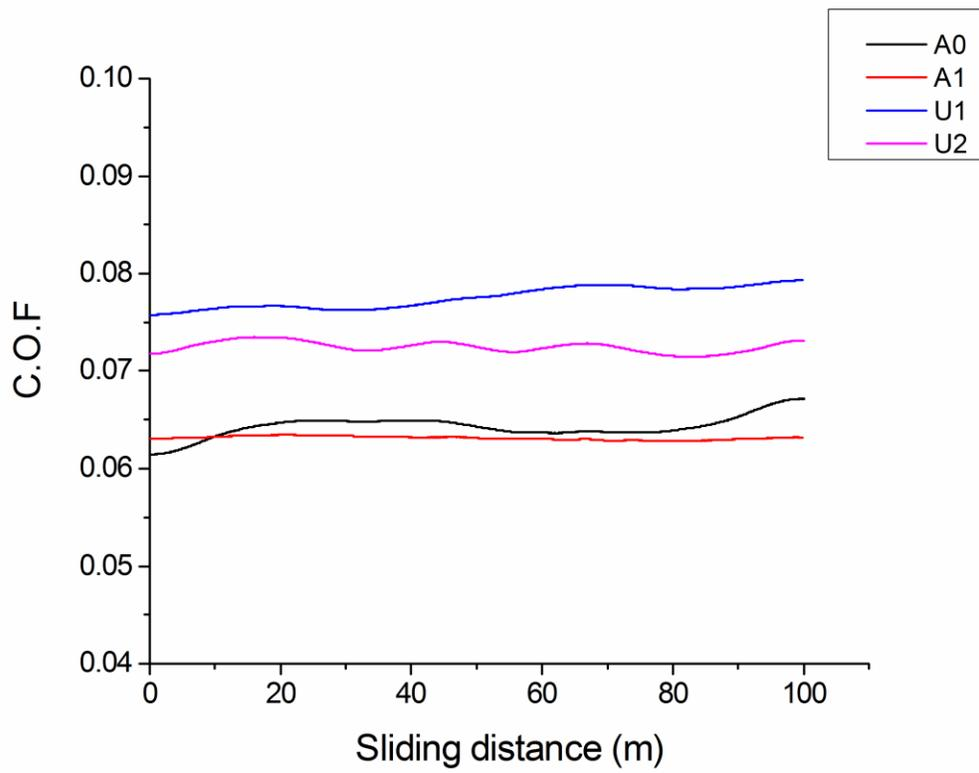
Figure 3. Dynamic COF curves of A0(as-prepared CPE treated sample), A1(CPE treated sample after polishing), U1(blank sample) and U2(sample with crosshatched surface).
