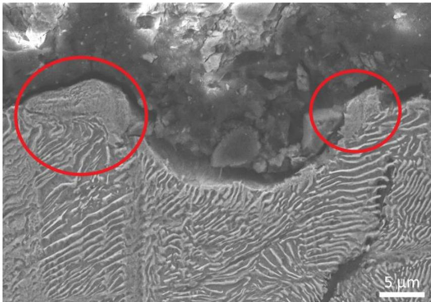
Figure 2. Cross-sectional structure of CPE treated sample showing the crater and re-solidification of iron.
