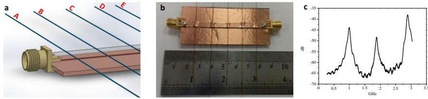
Figure 1. (a) 3D schema of the microfluidics/microwave device. (b) Picture of the microwave resonator. The dimensions of the glass slide are 2.5cm by 7.5cm. (c) The amplitude response of the sensor under spectrum analyzer.
