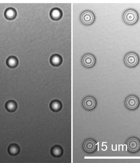
**Figure 5.** Top view optical microscopy images of blistering on a silica substrate (right) and de-wetting on an alumina substrate (left).  $\Omega \equiv p_{L,max}/p_{E,max} > 0(1)$
