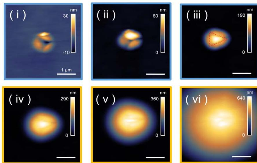
**Figure 3.** Two growth patterns of droplets beneath coatings observed by AFM. (i-iii) Growth with a fixed radius. (iv-vi) Growth with a fixed contact angle. The polymer used was a 33-nm thick CFx and the substrate was a polished silicon wafer (100).
