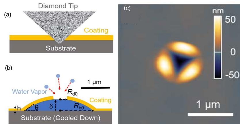
**Figure 2.** Schematic diagram of (a) indentation induced pinhole formation, and (b) pinhole induced blistering. (c) Height profile of the pinhole using AFM.
