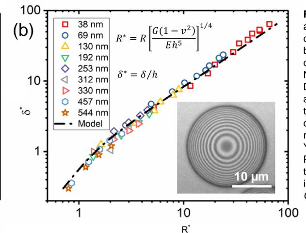
**Figure 7.** Radius and central deflection of blisters. (a) Raw data. (b) Normalized data. Dashed line: Plate and membrane theory. The shape of the blister is related to coating Young's modulus  $E$ , Poisson's ratio  $\nu$ , thickness  $h$ , and interfacial adhesion  $G$ .
