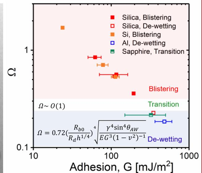
**Figure 6.** Blistering criteria map. With the same coating and pinhole geometry, substrate having high adhesion with the coating (sapphire, aluminum) showed de-wetting, while others showed blistering.
