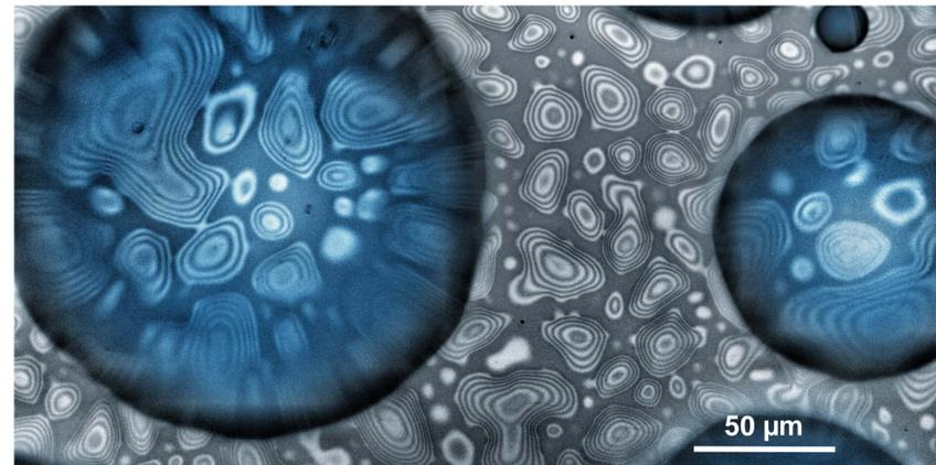
**Figure 1.** Water blisters on a 50-nm thick polystyrene film. The blisters are observable from the interferometric fringes. Water droplets on top of the coating are false colored blue.
