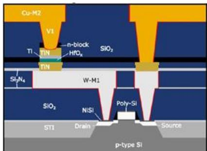
Fig.1: Schematic of CMOS-ReRAM integration.
