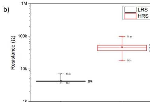
Fig. 4: a) Measured HRS and LRS for 50 1T1R cells, and b) Statistical variation of those parameters showing min, max along with inter-quartile range of all values for all cells tested.
