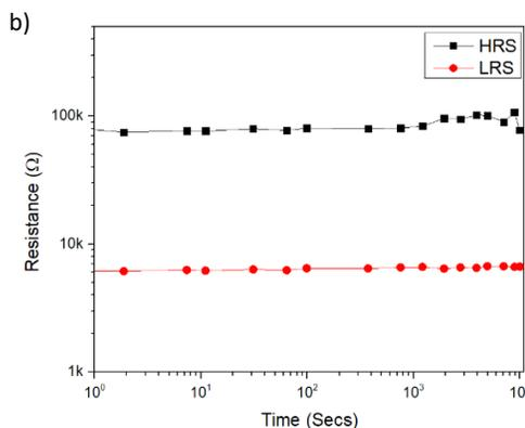
Fig. 5: a) Endurance measurement up to 1 billion switching cycles, and b) HRS and LRS retention up to  $10^4$  seconds at  $100^\circ\text{C}$ .
