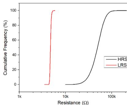
Fig. 6: Cumulative frequency distribution plot of LRS and HRS for fabricated HfO2 based RRAM devices.
