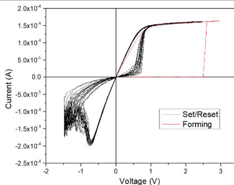
Fig. 2: Pulsed I-V sweeps showing set and reset operation of RRAM device.
