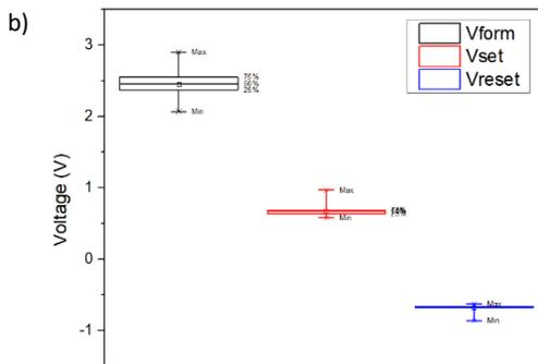
Fig. 3: a) Measured  $V_{form}$ ,  $V_{set}$  and  $V_{reset}$  for 50 1T1R cells, and b) Statistical variation of those parameters showing min, max along with inter-quartile range of values for all cells.
