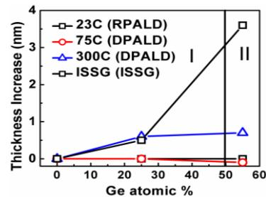
Figure 2. ISSG exhibits a stronger oxidation with increasing Ge concentration than ALD. ALD also shows enhanced oxidation at higher temperature (> 300 °C). 75 °C PEALD has minimal oxidation with good quality oxide.
