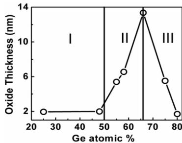
Figure 1. ISSG oxidation of SiGe films exhibits three types of behavior: (I) slow oxidation, (II) fast oxidation with condensation, and (III) sublimation. We can explain this behavior with a binary mixing model [5].
