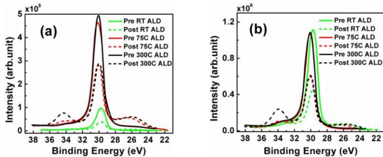
Figure S3.  $\text{Ge}^{3d}$  spectra using XPS for (a)  $x = 0.25$  and (b)  $x = 0.55$   $\text{Si}_{1-x}\text{Ge}_x$  films before and after PEALD oxide deposition at room temperature, 75 °C and 300 °C. For both  $x = 0.25$  and 0.55, a  $\text{GeO}_x$  peak is observed at ~34 eV, which increases with temperature. Interestingly,  $\text{GeO}_x$  can be formed with low temperature PEALD processes [2]. This behavior is not observed with ISSG processes at  $x = 0.25$  (see Figure S2(a)).
