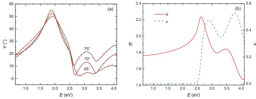
**Fig. 1** (a) Experimental (green dashed line) and best-model (red solid line)  $\Psi$ -spectra for a  $\text{Si}(\text{bzimpy})_2$  thin-film sample measured at three different angles of incidence  $\Phi_a = 65^\circ, 70^\circ$ , and  $75^\circ$  in spectral range from 0.65 eV to 4.1 eV. An excellent agreement between the experimental and best-model calculated data is obtained using the optical constants shown in Fig. 1(b).
