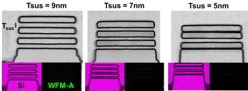
Fig. 1: TEM micrographs (*inset*: EDS map of Si, WFM-A) post gas phase dry etch of WFM-A. TEMs show structural feasibility post etch and EDS confirming complete etch of WFM-A. Si channel collapse at  $T_{sus} = 5\text{nm}$  can be explained from TEM sample preparation.
