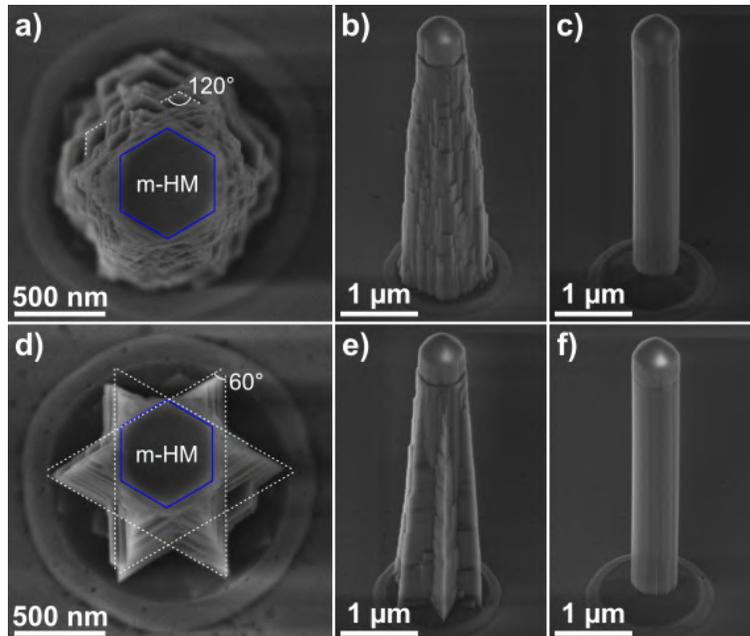
Figure 2. a), b), c) KOH 44% wet treatment on AlN pillars of 500 nm diameters: a), b) top view, and tilted view after a partial wet etching (20 sec), respectively, c) complete wet etching (360 sec). d), e) f) KOH 5% wet treatment on AlN pillars of 500 nm diameters: a), b) top view, and tilted view after a partial wet etching (2 min), respectively, c) complete wet etching (20 min).
