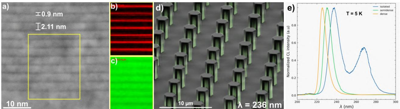
Figure 3. AlGaIn QW's on a 2  $\mu\text{m}$  diameter pillar: a) TEM HAADF image, b), c) TEM EELS signal indicating the presence of Gallium and Aluminium respectively. d), e) Cathodoluminescence image and spectra showing the UV-C emission.
