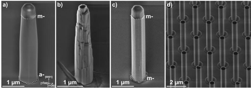
Figure 1. a), b), c) GaN pillars of 500 nm diameter with a m-oriented HM after plasma etching, KOH wet etching without HM, and KOH wet etching with the HM, respectively. d) Arrays of 500 nm GaN pillars after the best process (plasma etching, KOH with HM, HM removal using fluorhydric acid).
