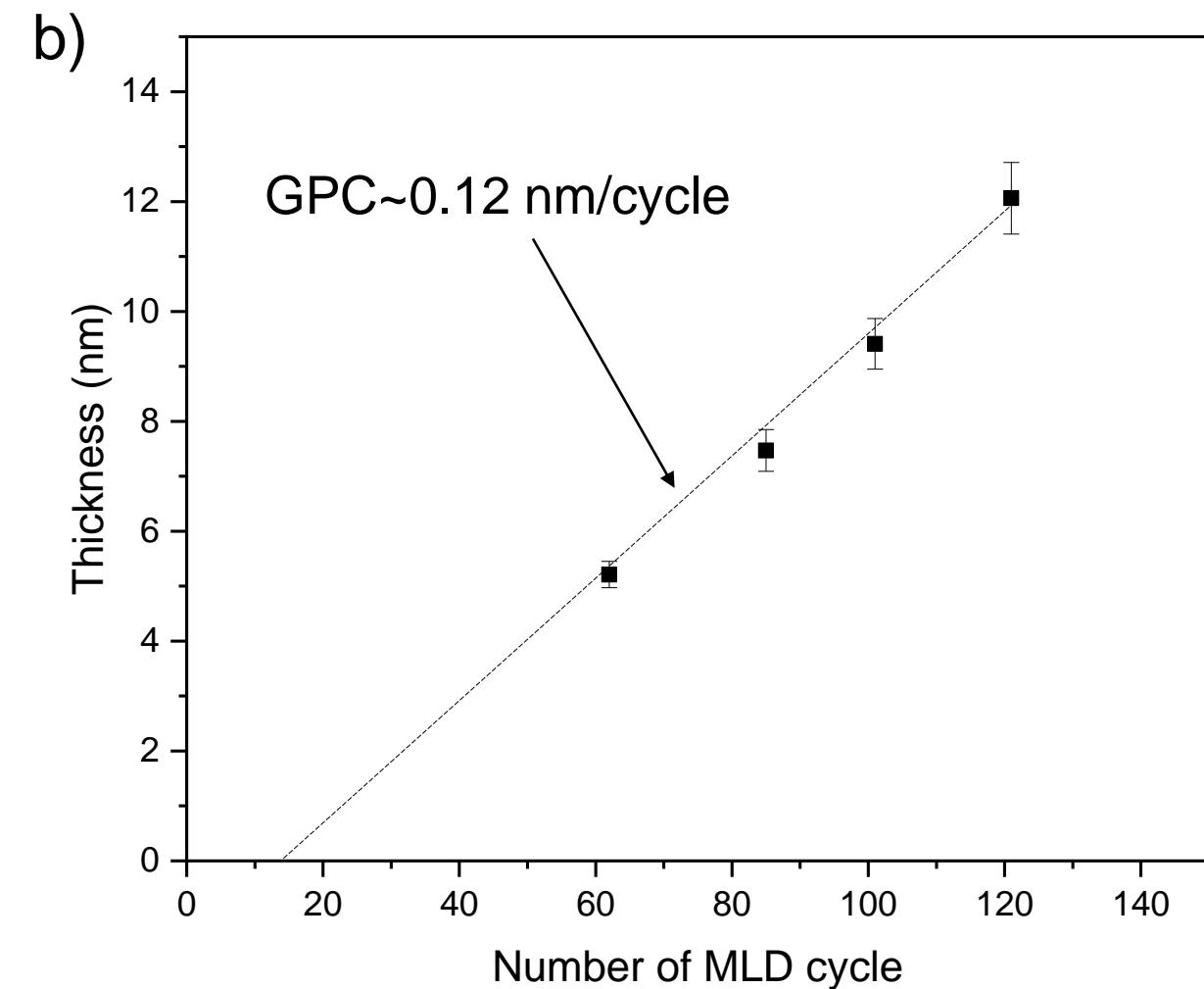
**Figure 1.** **a)** Growth per cycle (GPC) versus AC pressure and **b)** film growth at the 4 doses (50sccm BB). #% is percentage of surface roughness (rms) over thickness.
