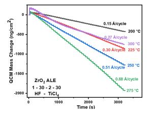
Figure 1. Mass changes during ZrO<sub>2</sub> ALE cycles at 200, 225, 250, 275, and 300 °C with the HF and TiCl<sub>4</sub> with 1–30–2–30 at pressures of 0.1 Torr for HF and 0.13 Torr for TiCl<sub>4</sub>.
