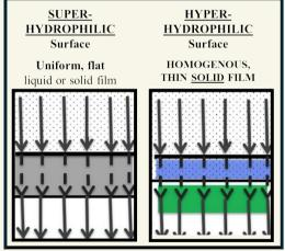
Fig. 4 Illustrates the difference between water condensation on superhydrophilic surfaces and hyper-hydrophilic surfaces. In the new hyperhydrophilic surfaces, water is absorbed by the coating allowing the surface to collect more water during condensation without dissolution of the coating.
