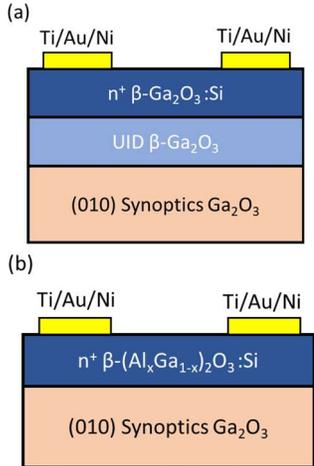
Figure 1 – Schematic of fabricated test structures on (a)  $\beta\text{-Ga}_2\text{O}_3$  (b)  $\beta\text{-(Al}_x\text{Ga}_{1-x})_2\text{O}_3$
