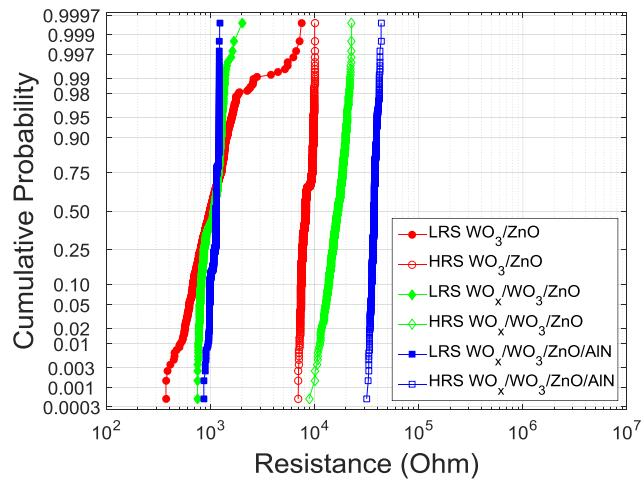
The high resistance state (HRS) and low resistance state (LRS) of 1000 cycles in  $\text{WO}_3/\text{ZnO}$ ,  $\text{WO}_x/\text{WO}_3/\text{ZnO}$ , and  $\text{WO}_x/\text{WO}_3/\text{ZnO}/\text{AlN}$  ReRAM. With the  $\text{WO}_x$  layer, the ReRAM endurance can extend to  $10^4$  cycles. The AlN film stabilizes the HRS and increase the resistance ratio.
