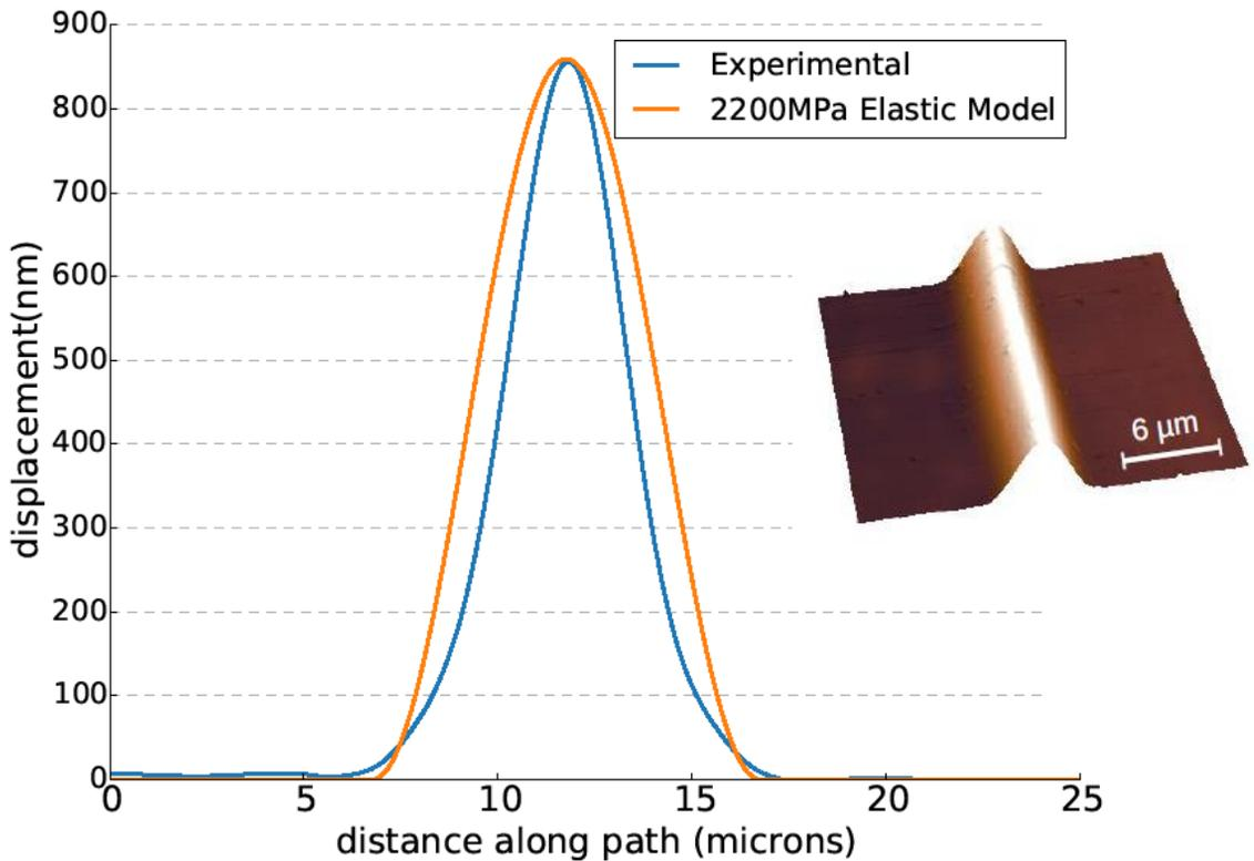
**Figure 2:** (right ) 3D Atomic force microscopy micrograph of characteristic buckling structures observed on a 400 nm thick gold film deposited on a silicon substrate ; (left ) Difference between the experimental profile and a numerical profile obtained with a pure elastic linear model.
