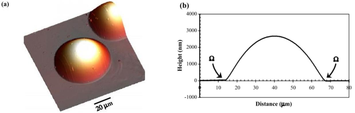
**Figure 1:** Figure 1: (a) 3D Atomic force microscopy micrograph of a circular buckle structure observed on a 600 nm thick gold film deposited on a silicon substrate (b) Cross section of the blister; A strong bending  $\Omega$  on the edge of the buckling structure is observed (from Coupeau et al., 2004).
