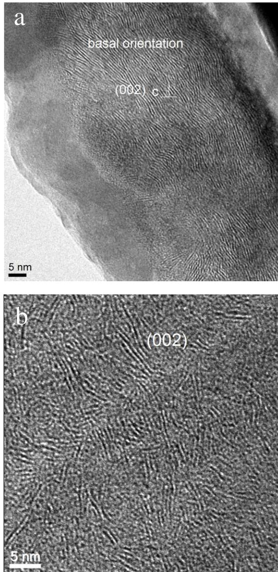
Fig.1. TEM images: a) Pure WS<sub>2</sub> showing clear basal orientation; b) WS<sub>2</sub>/a-C coating showing WS<sub>2</sub> platelets randomly distributed in amorphous carbon matrix.
