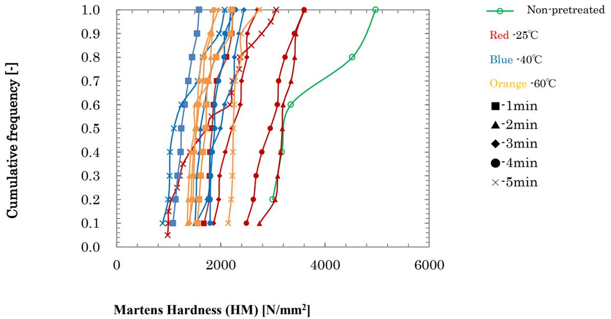
Figure 1 Cumulative frequency of martens hardness of non-pretreated and treated WC-Co surface. WC-Co substrates are measured with 200 gf.
