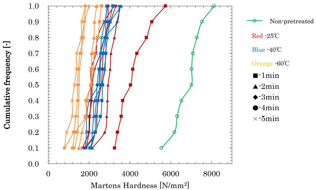
Figure 2 Cumulative frequency of martens hardness of non-pretreated and treated WC-Co surface. WC-Co substrates are measured with 25 gf.
