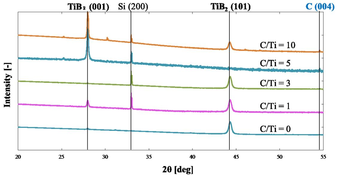
Figure 1 XRD results of as-deposited TiBC thin films with different C/Ti ratio.
