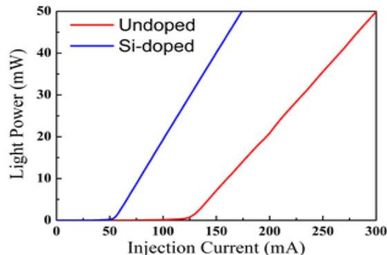
Figure 1 Single-side CW P-I curves of the two QD lasers
