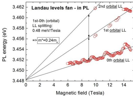
Fig. 5: Landau level fan obtained from evaluation of magneto-PL data (c.f. Fig. 1). From the separation of the LLs an effective electron mass of  $0.24 m_0$  is extracted.
