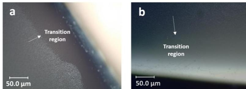
Fig. 1: Representative Nomarski images of the grown layers on a) (111)B and b) (111)A substrates at optimum growth conditions taken at the wafer edge.
