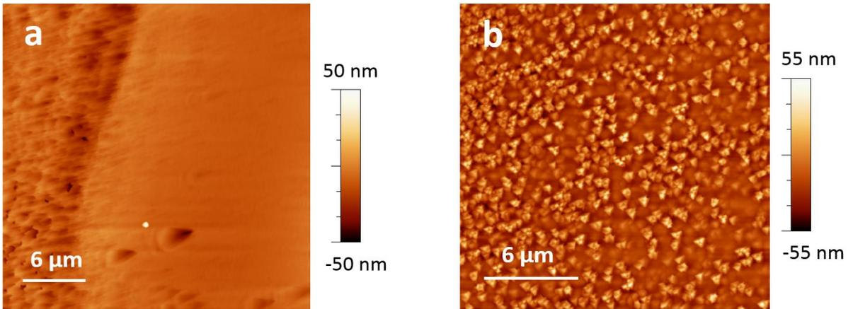
Fig. S.1: AFM height mode images of the grown epilayers on the exact a) (111)B and b) (111)A. The panel (a) shows the transition between the rough and smooth regions.
