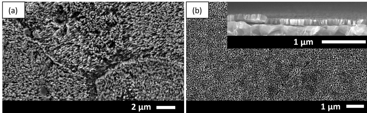
Figure 1: Plan view SEM images of GaN nanowires on (a) a Ti foil and (b) an amorphous foil, inset shows cross section view of the wires on the amorphous foil.
