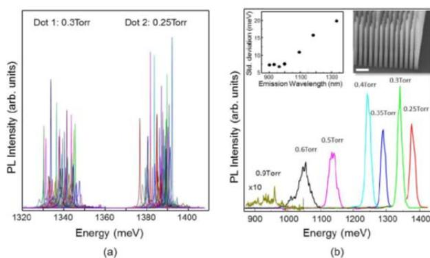
**Figure 4** (a) PL spectra from 50 double dot nanowires. (b) PL spectra from nanowire arrays with dots grown using different AsH<sub>3</sub> flux. Right inset show an SEM image of one of the arrays (scale bar is 1 μm). Left inset shows the energy spread dependence on emission wavelength.
