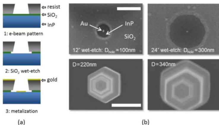
**Figure 3** Processing steps for the preparation of the growth substrate. (b) Upper panel:  $\text{SiO}_2$  hole opening for different etch times. Lower panel: top-view SEM of nanowires grown in the different size openings. Scale bars are 200 nm.
