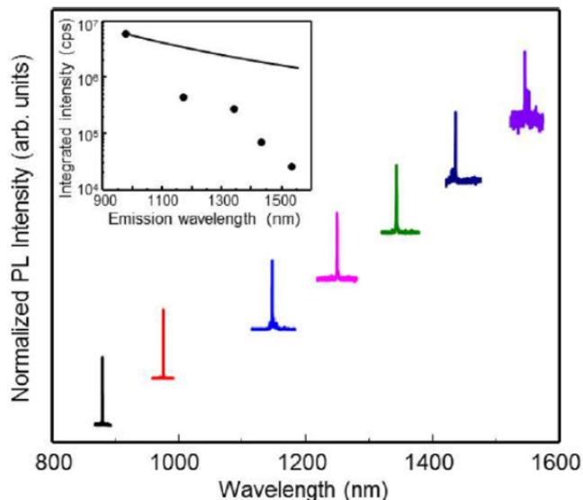
**Figure 6** Normalized PL spectra of single InAsP/InP nanowire quantum-dot emitters in tailored photonic waveguides. Inset shows the emission-wavelength dependence of the count rate at the first lens (circles) as well as that of a radiating dipole (line).
