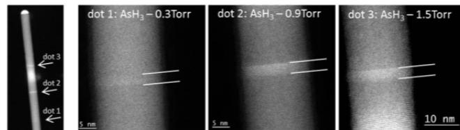
**Figure 2** HAADF TEM image of a nanowire containing three dots grown under different AsH<sub>3</sub> flux.
