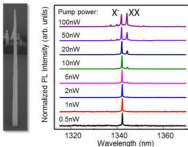
**Figure 1** Power-dependent spectra for a dot with a charged exciton ground-state emission  $\lambda = 1342$  nm
