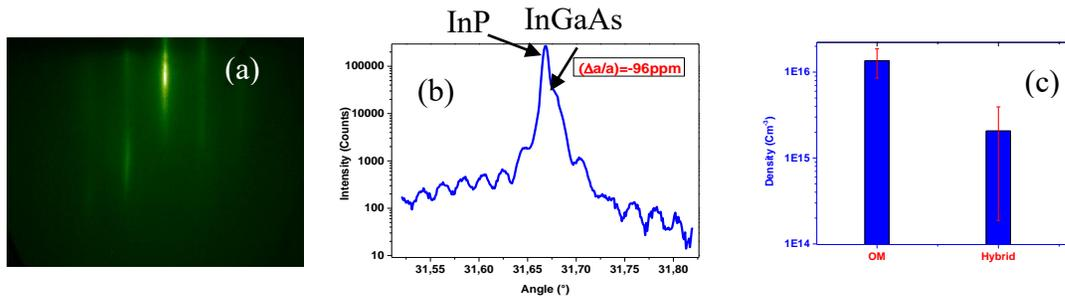
Fig. 1: (a) and (b) RHEED patterns of and HRXRD for InGaAs grown by Hybrid MBE-CBE respectively. (c) Background density of undoped InGaAs grown by standard CBE and hybrid.MBE-CBE.
