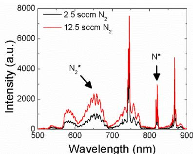
Figure 1. OES of a plasma discharge with low and high flow rates of  $\text{N}_2$ .
