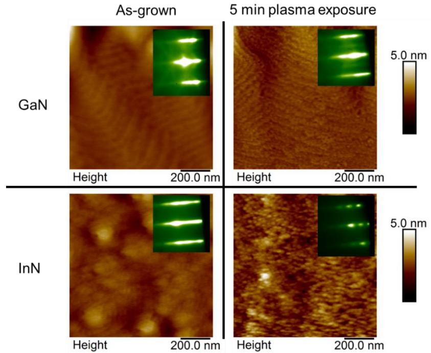
Figure 3. AFM and RHEED insets of GaN and InN surfaces as-grown and after 5 minutes of plasma exposure. InN films are more sensitive to plasma exposure and exhibit rougher surfaces compared to the GaN films.
