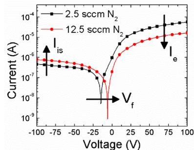
Figure 2. Langmuir probe current-voltage characteristics of a plasma with low and high flow rates of  $\text{N}_2$ .
