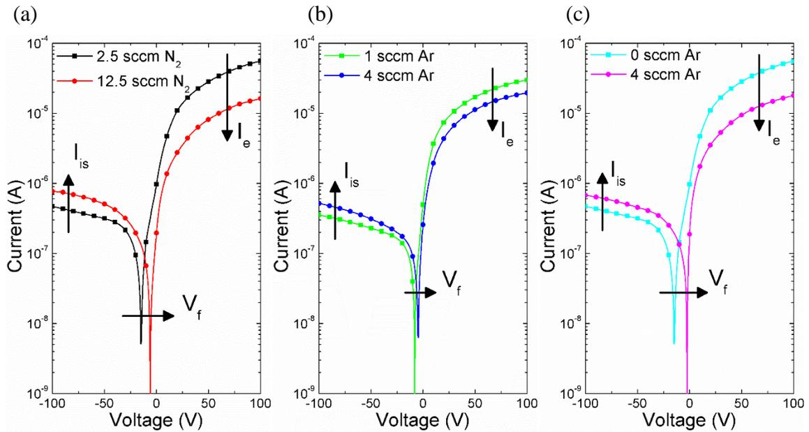
Figure 4. Langmuir probe current-voltage characteristics of a plasma operated at 350 W: (a) pure nitrogen flows, (b) pure argon flows, and (c) mixed chemistry of argon flows with a constant 2.5 sccm nitrogen flow.
