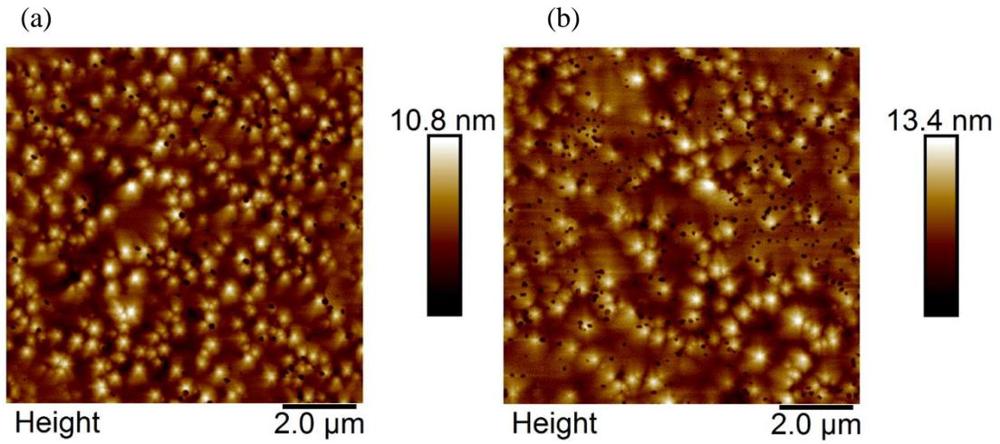
Figure 5.  $10 \times 10 \mu\text{m}^2$  AFM images of  $1 \mu\text{m}$ -thick InN surfaces grown via MME with a plasma power of (a) 350 W and (b) 550 W. Pit density is increased at higher plasma powers.
