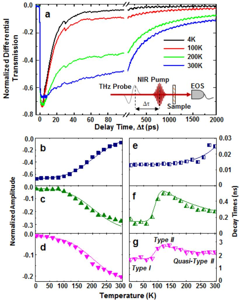
Figure 3: Carrier dynamics of the multiple QW system: (a) Normalized differential THz transmission for a range of lattice temperatures. The inset shows the collinear experimental geometry of the THz probe and near-infrared (NIR) pump. (b) - (d) and (e) - (g) are the amplitude and decay times of the fast, intermediate, and slow carrier dynamics extracted from fitting the transients. In (g), the regions of type-I, type-II and quasi-type II behavior are labeled.
